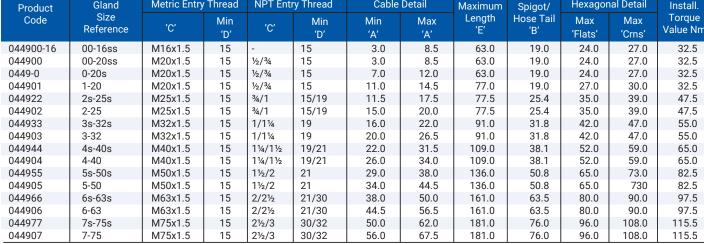
All dimensions except NPT are in mm. Intermediate thread sizes are available on request.NPT threads should be tightened 'wrench tight'.
