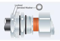
If the gland has NPT entry threads fitted to a threaded entry then IP68 (2m) can be achieved by applying one of the following tested and approved grease types to the thread:- Renolit Lubrene CA700 or LX220 EP2, Renolit LC-WP2 or Moly LX2, or Dow Corning 4 Electrical Insulating Compound.
