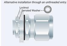
If the apparatus is untapped use a locknut.
