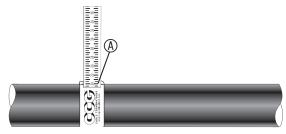
For accurate sizing, use a CCG Dimension Tape (4) on the outer cable sheath.
