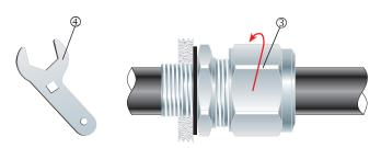
5. Tighten the outer nut ③ to the installation torque using a CCG Spanner ④ to produce a seal and grip on the cable.
