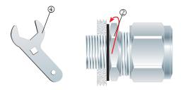
Screw the inner ② into the apparatus. Tighten the inner ② to the installation torque using a CCG Spanner ④
