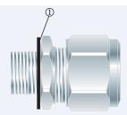
To maintain IP66/68, ensure the gasket ① is in place.
