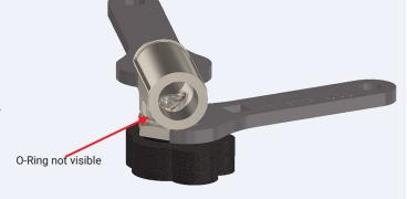
Check that the O-ring seal is not visible (this ensures that the required number of threads are engaged in the equipment). If the O-ring is visible then repeat steps 1 to 4 correctly.
