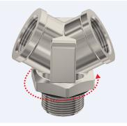
Ensure that the threaded entry on the equipment has a flat, square surface to engage the sealing gasket. Tighten the adaptor, complete with sealing gasket, into the equipment until it is fully secured noting the maximum torque figures in the table overleaf.
