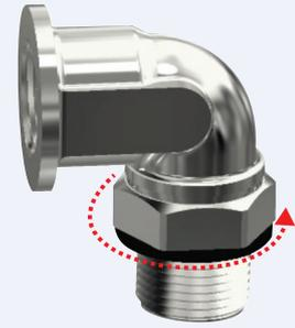
2. Ensure that the threaded entry on the equipment has a flat, square surface to engage the sealing gasket. Tighten the adaptor, complete with sealing gasket, into the equipment until it is fully secured noting the maximum torque figures in the table overleaf.
