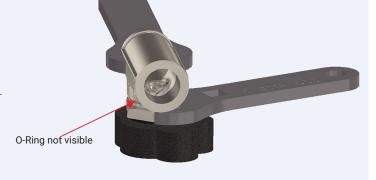
Check that the O-ring seal is not visible (this ensures that the required number of threads are engaged in the equipment). If the O-ring is visible then repeat steps 1 to 4 correctly.
