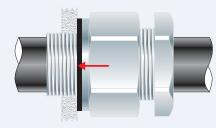
Pass the cable end through the gland assembly.
