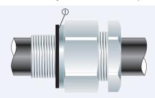
2. To maintain IP66/68, ensure the gasket  ${\mathfrak Q}$  is in place.
