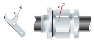
Screw the inner ② into the apparatus. Tighten the inner ② to the installation torque using a CCG Spanner 4
