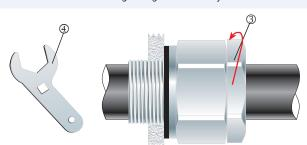
Tighten the outer nut ③ to the installation torque using a CCG Spanner ④ to produce a seal and grip on the cable. 100% Cable retention load. No additional clamping required.
