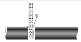
For accurate sizing, use a CCG Dimension Tape (A) on the outer cable sheath.
