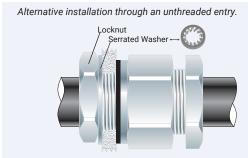
If the apparatus is untapped use a locknut.
