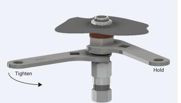
4. Hold the body of the breather / drain adaptor with a spanner when tightening a cable gland into the female thread.
