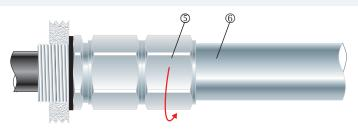
5. Fit the threaded conduit end 6 into the female rotating threads 5 as indicated.
