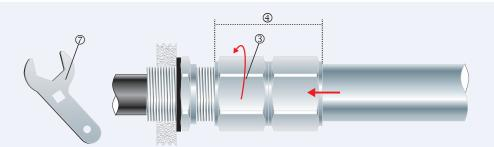
4. Pass the cable end through the conduit assembly ④ and the gland assembly. Tighten the outer ③ to the installation torque using a CCG Spanner ⑦ to produce a seal and grip on the cable.
