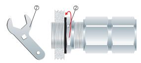
3. Screw the gland unit into the apparatus. Tighten the inner until hand tight 2 using a CCG Spanner 2 with ¼ turn.
