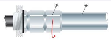
5. Fit the threaded conduit end <sup>(6)</sup> into the female rotating threads <sup>(5)</sup> as indicated.
