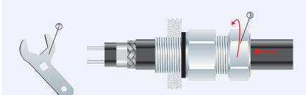
4. Pass the cable end through the conduit assembly and the gland assembly. Tighten the outer ③ to the installation torque using a CCG Spanner ⑦ to produce a seal and grip on the cable.
