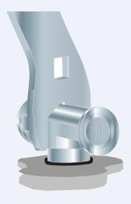
3. Ensure the T Adaptor is securely positioned and hold the adaptor flats using a CCG Spanner whilst fitting cable glands to the female threads.
