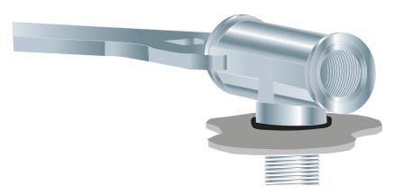
2. If fitting to a clearance hole, secure the T Adaptor using a locknut. (Use a serrated washer and locknut in high vibration areas.)
