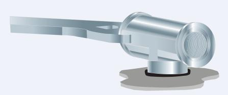
1. Ensure that the threaded entry on the equipment has a flat surface to engage the sealing gasket. Tighten the T Adaptor, complete with sealing gasket, into the equipment using a spanner until it is fully secured, noting the maximum torque figures in the table overleaf.
