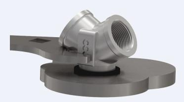
1. Ensure that the threaded entry on the equipment has a flat surface to engage the sealing gasket. Tighten the Y Adaptor, complete with sealing gasket, into the equipment using a spanner until it is fully secured, noting the maximum torque figures in the table overleaf.
