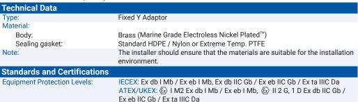
NMETRO: Ex db I Mb, Ex eb I Mb, Ex db IIC Gb, Ex eb IIC Gb, Ex tb IIIC Db
