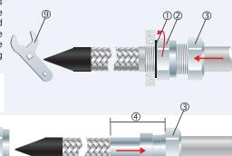
Unscrew the outer nut ③. Withdraw the cable and resin sleeve / insert sub-assembly ④ Remove the resin sleeve \$ from the sub-assembly 4, leaving the resin-retaining seal 6 in place. Remove the tape from the end of the braid.
