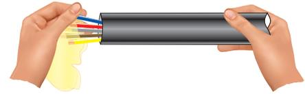
2. Using insulation tape, bundle the cores together at the end.
