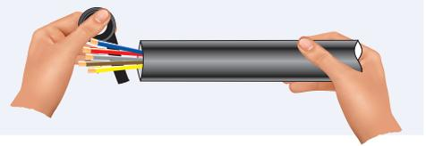
3. To maintain IP66/68, ensure that the gasket ① is in place. Screw the gland unit into the apparatus and tighten the inner ② using a CCG spanner ⑤. Slacken, but do not remove, the outer seal nut ④. Pass the cable end through the outer seal nut ④ and push the bundled cable cores through the gland, taking care as it passes through the protective resin pot ⑧. Once the cable is correctly positioned, tighten the outer seal nut ④ to the recommended installation torque.
