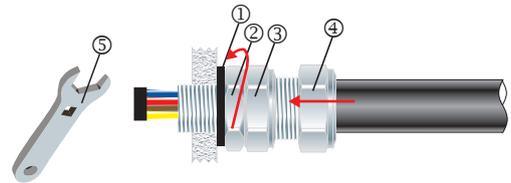
If the gland has NPT entry threads fitted to a threaded entry then IP68 (2m) can be achieved by applying one of the following tested and approved grease types to the thread:- Renolit Lubrene CA700 or LX220 EP2, Renolit LC-WP2 or Moly LX2, or Dow Corning 4 Electrical Compound.
