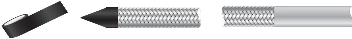
3. Wrap insulation tape over and around the end of the screen to prevent the screen from being displaced as the cable is fitted to the gland. The insulating tape should form a gradual taper to assist with passing the cable through the internal earthing device.
