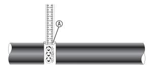
For accurate sizing, use a CCG Dimension Tape (4) on the outer cable sheath.
