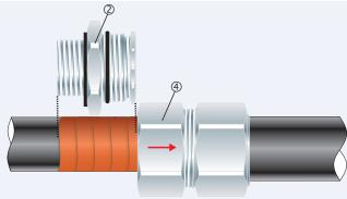
2. Screw the body ④ off and pass the cable end through the body ④. Cut the PVC sheath exposing the copper tape to the length of the inner ②.
