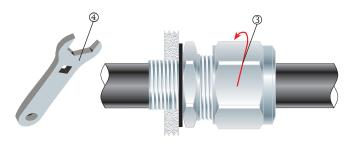
5. Tighten the outer nut  $\@3$  to the installation torque using a CCG Spanner  $\@4$  to produce a seal and grip on the cable.
