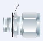
2. To maintain IP66/68, ensure the gasket ① is in place.
