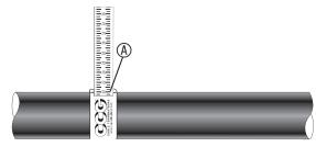
For accurate sizing, use a CCG Dimension Tape (A) on the outer cable sheath.
