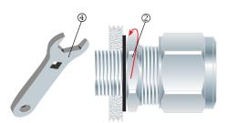
Screw the gland unit into the apparatus. Tighten the inner ② to the installation torque using a CCG Spanner 4.
