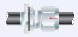
4. Pass the cable end through the gland assembly.
