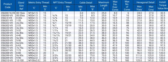
All dimensions except NPT are in mm. Intermediate thread sizes are available on request. NPT threads should be tightened 'wrench tight'.
