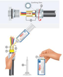
5. Re-insert the barrier pot sub-assembly 4 back into the inner 2.
