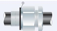
2. To maintain IP66/68, ensure the gasket  ${f D}$  is in place.
