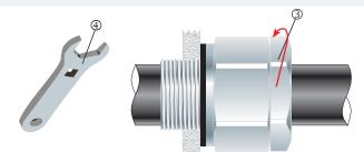
5. Tighten the outer nut ③ to the installation torque using a CCG Spanner ④ to produce a seal and grip on the cable. 100% Cable retention load. No additional clamping required.
