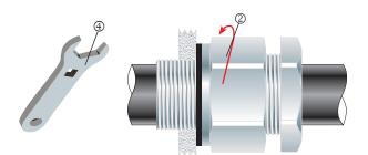
3. Screw the inner 2 into the apparatus. Tighten the inner 2 to the installation torque using a CCG Spanner 4.
