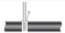
1. For accurate sizing, use a CCG Dimension Tape (1) on the outer cable sheath.
