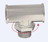
Ensure that the threaded entry on the equipment has a flat, square surface to engage the sealing gasket. Tighten the adaptor, complete with sealing gasket, into the equipment until it is fully secured noting the maximum torque figures in the table overleaf.
