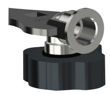
3. Ensure the adaptor is securely positioned and hold the adaptor flats using a spanner whilst fitting a cable gland to the female thread.
